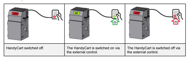
The HandyCart can also be switched off/on via its own membrane switch panel. (To this end it is necessary to separately switch on the external control.)
